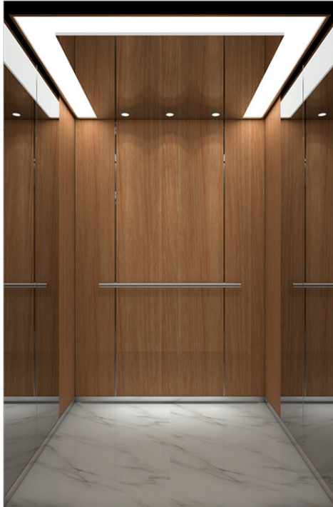
FJ-K142 Optional Ceiling: Mirror stainless steel + acrylic + LED downlights + decoration veneer steel Rear wall: Wood veneer + mirror stainless steel strip Side wall: Wood veneer + mirror stainless steel Front wall: Hairline stainless steel Handrail: Hairline stainless steel round Floor: PVC / Marble (optional)
